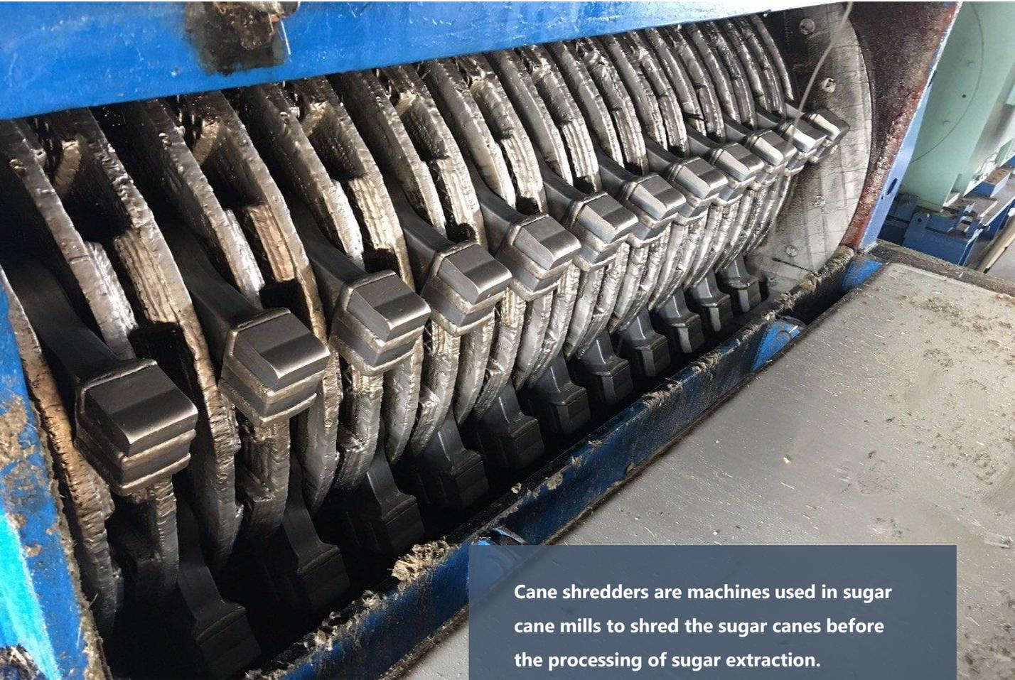
Cane shredders are machines used in sugar cane mills to shred the sugar canes before the processing of sugar extraction.
