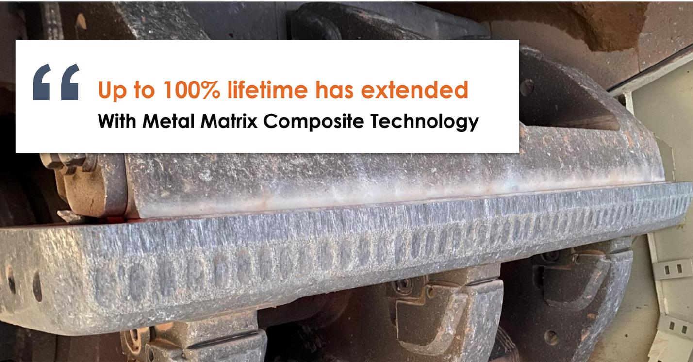
No one type of material is able to suit all impact crushing applications. It is very important to choose the right material for blow bar for the right application.
