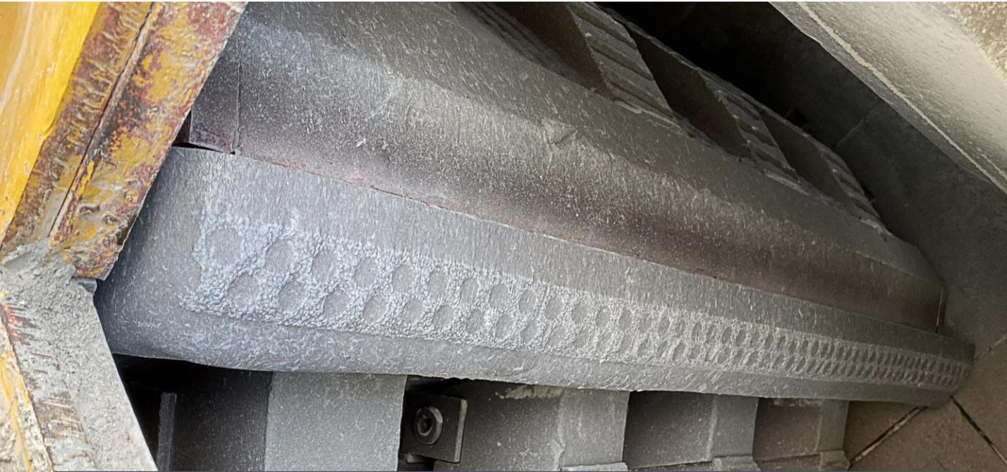
Blow bar is a crucial wear part on impact crusher. The good blow bars and right material options are so important to keep the crusher running safely and cost efficiently.
