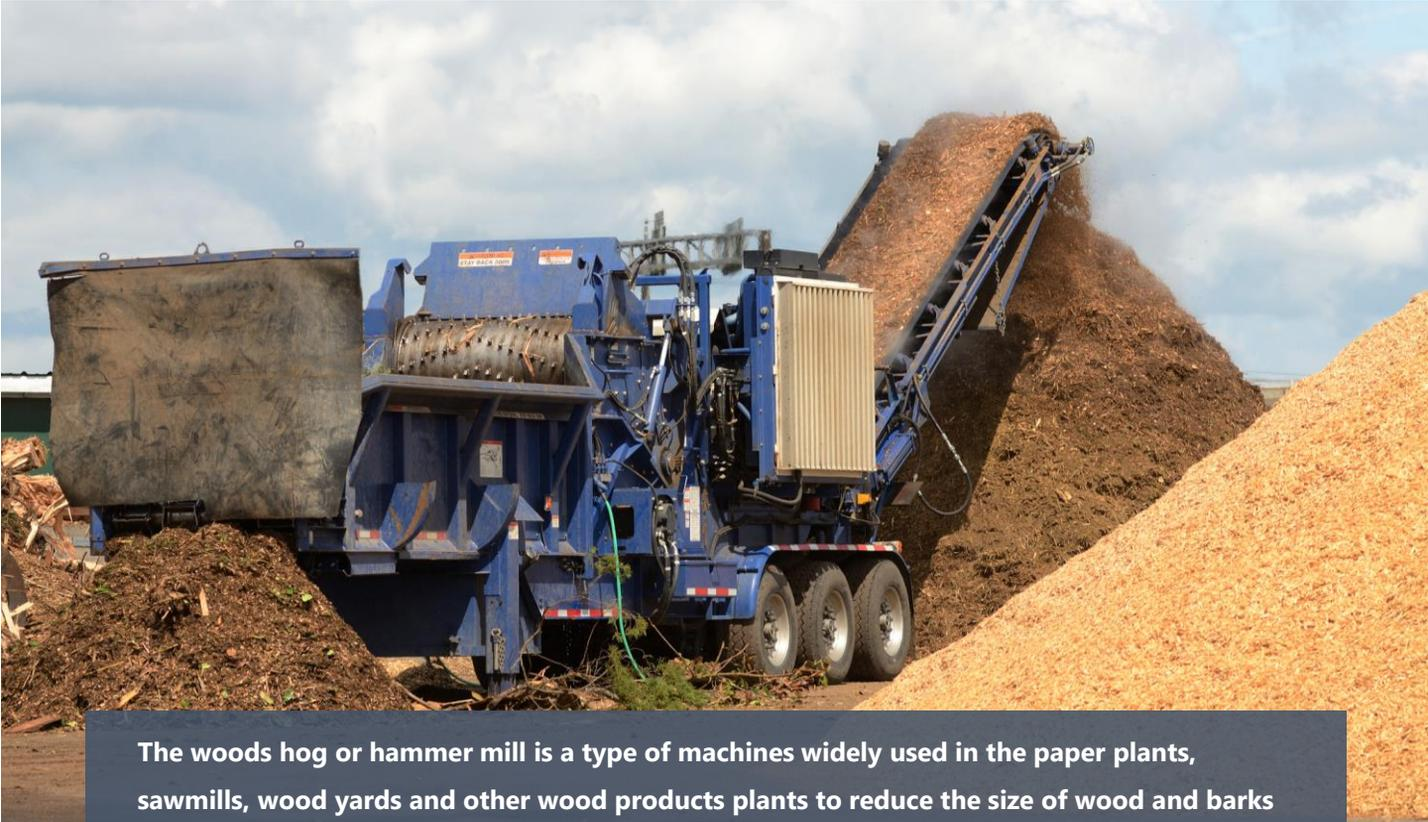
The woods hog or hammer mill is a type of machines widely used in the paper plants, sawmills, wood yards and other wood products plants to reduce the size of wood and barks for preparation of next process. It mainly consists of housing, shaft, rotor and other accessories. Hammers including tips are the main wear parts on the machine and Sunwill can supply them with the following options for materials:
